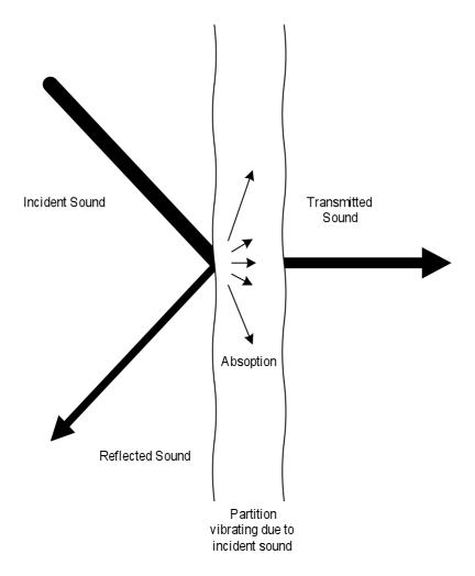
The measure used is the absorption co-efficient which is, basically, a co-efficient between 0 and 1 relating to the proportion of sound that is absorbed. A co-efficient of 1 means that there is no reflected sound.
